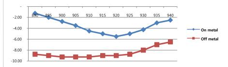
•FASTENER reads longer by 30% or less off metal (or on non metal surface). It can be applied for BOTH metal and off metal application.
